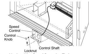
Figure 32 - Attaching Speed Control to Firebox
